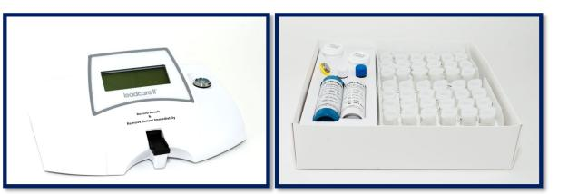
The LeadCare II instrument, along with the consumables provided in each test kit.
